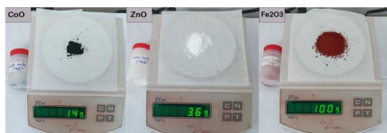
Figure 2(b) Experimental procedure of Cobalt Zinc Ferrite nanoparticle were prepared by stoichiometric proportion ( \text{Co}_{0.3}\text{Zn}_{0.7}\text{Fe}_2\text{O}_4 )
