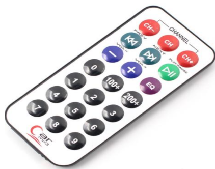
( a ) IR remote control transmitter
