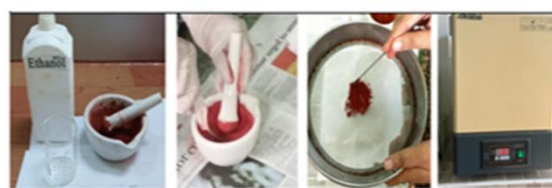
Figure 2(d) Grinding starting materials with ethanol and sintering temperature at 1000^\circ\text{C} for 4 hours
