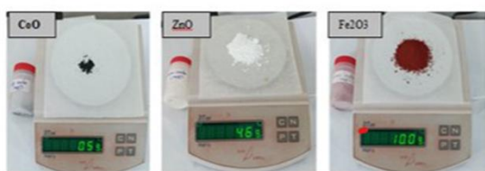
Figure 2(a) Experimental procedure of Cobalt Zinc Ferrite nanoparticle were prepared by stoichiometric proportion ( \text{Co}_{0.1}\text{Zn}_{0.9}\text{Fe}_2\text{O}_4 )
