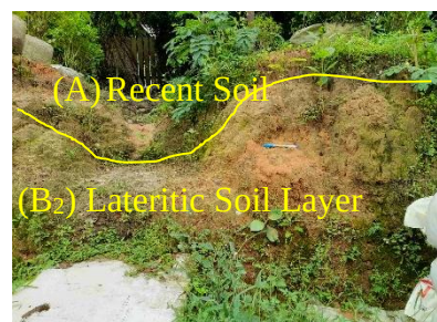
Figure (16) The two layers of lateritic soil outcrop exposed at Location (12)
