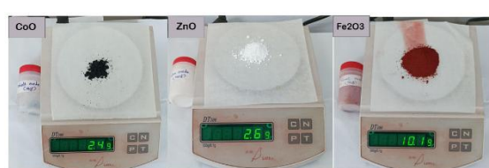
Figure 2(c) Experimental procedure of Cobalt Zinc Ferrite nanoparticle were prepared by stoichiometric proportion ( \text{Co}_{0.5}\text{Zn}_{0.5}\text{Fe}_2\text{O}_4 )
