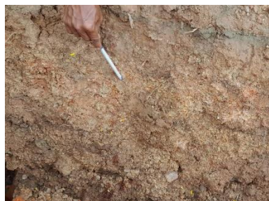
Figure (14) B 2 layers of lateritic soil outcrop exposed at Location (10)
