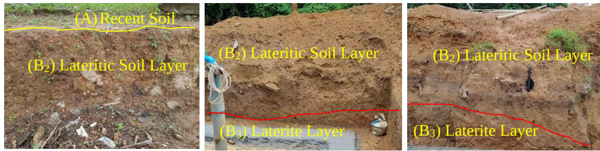
Figure (20) The two layers of lateritic soil outcrop exposed at Location (20) Figure (21) The two layers of lateritic soil outcrop exposed at Location (21) Figure (22) The two layers of lateritic soil outcrop exposed at Location (21)
