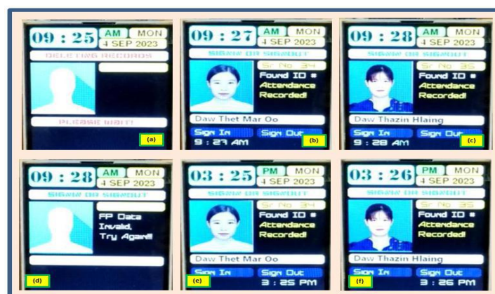
Figure 7. (a) Clearing EEPROM memory on the start of a week (Monday) (b) Sign in for ID No.34 at 9:27 AM (c) Sign in for ID No.35 at 9:28 AM (d) Fingerprint did not match for incorrect position (e) Sign out for ID No.34 at 3:25 PM (f) Sign out for ID No.35 at 3:26 PM
