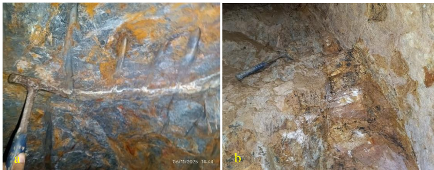
Figure 3. Photo showing (a) Veinlets and stringers system of sulfide quartz vein in mudstone, (b) individual vein system of sulfide quartz vein in sandstone
