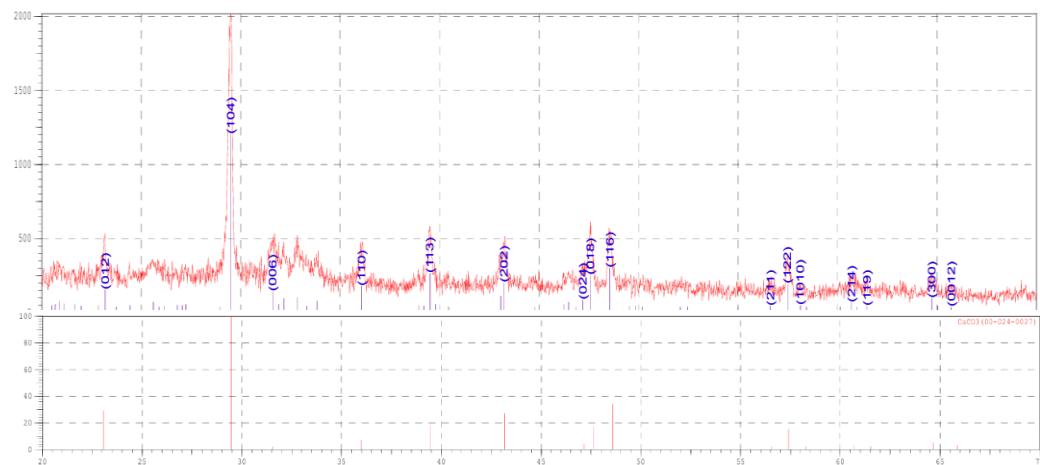
Figure 3 (c) XRD pattern of blackgram waste activated carbon at 500 °C
