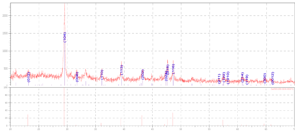
Figure 3 (b) XRD pattern of blackgram waste activated carbon at 400 °C
