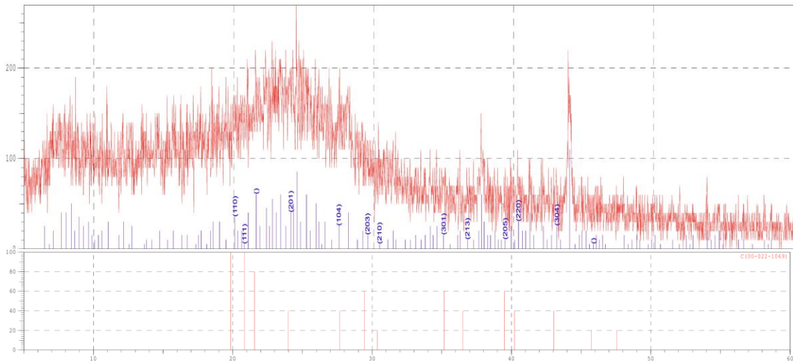
Figure 6 XRD pattern for corn husk biochar at 400 °C
