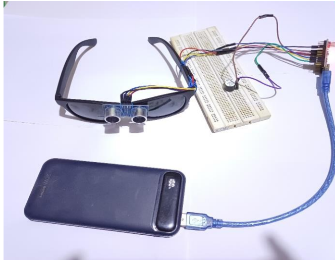
Figure 11. The photograph of the whole circuit connection system with the power bank
