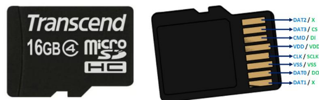
Figure 5. Pinout diagram of a micro SD card
