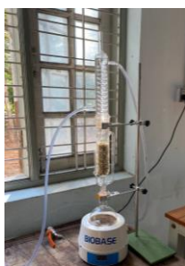
Figure 1 Extraction of Essential Oil by Soxhlet Extractor
